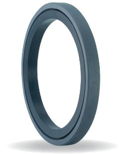
Merkel Omegat OMK-S is a two-piece seal set for sealing pistons, consisting of a PTFE profile ring and an elastomer Profile ring as a pre-stress element.
