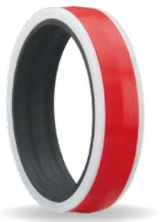
**Merkel Kompaktdichtung T 42** is a double-acting piston seal with a sealing element made of polyurethane, an elastomer activating element and two back rings.
