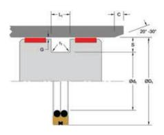
Applications with maximum radial clearance that are using nylon, phenolic, or PTFE bearings must ensure proper clearance in accordance with the bearing recommendations to avoid metal-to-metal contact. Please refer to Hallite Type 87, Type 506, and Type 533 Specification Sheets for this information.
