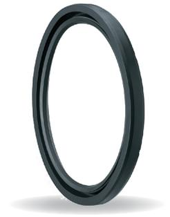
Merkel Radiamatic R37 is a radial shaft seal consisting of a fabric reinforced section of sturdy design, firmly bonded to the rubber sealing lip. A helical tension spring assists radial contact pressure of the lip on the shaft.
