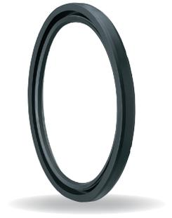
Merkel Radiamatic RS85 is a self-retaining shaft seal consisting of two different rubber compounds and an integrated steel band. The tension spring supports the radial force on to the shaft.
