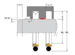
Applications with maximum radial clearance that are using nylon, phenolic, or PTFE bearings must ensure proper clearance in accordance with the bearing recommendations to avoid metal-to-metal contact. Please refer to Hallite Type 87, Type 506, and Type 533 Specification Sheets for this information.
